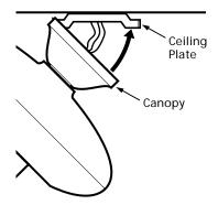
Figure 5a - Attaching Canopy to Ceiling Plate
